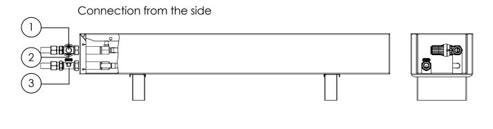
(1) Thermostatic valve, axial
